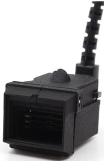
For untethered recordings, power (3.7 – 5V) must be supplied through the HDMI connector on the system using the SpikeGadgets power adaptor. Typically, a 3.7V rechargeable lithium battery is used. Also, a microSD card that has been formatted using the SpikeGadgets Logger Dock must be inserted into the SD card slot of the headstage. Once power is supplied, a set of possible LED indication patterns on the headstage signify system state:
