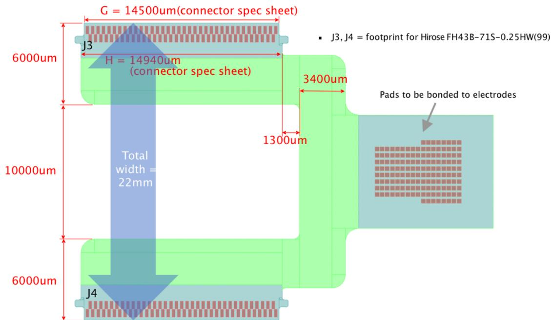
Figure 2- Flexible PCB routing the channels between the probe and the 128-channel modules
