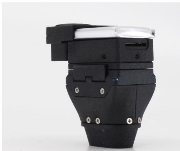
Figure 12 Neuropixels Headstage with battery
