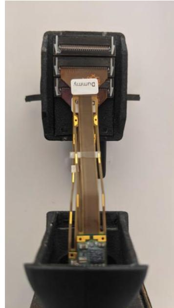
Figure 4 Probe and cone connection to the headstage
