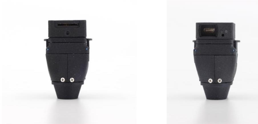
*Figure 1 Front and back view of Neuropixels Headstage*
