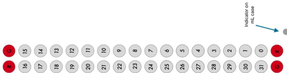
Figure 4- Pin out for 32-channel logger bottom
