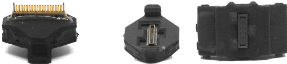
Figure 5- miniLogger 32 base with 36-pin Omnetics connector, Figure 6- miniLogger 32 base and processor base with 40-pin Hirose connector
