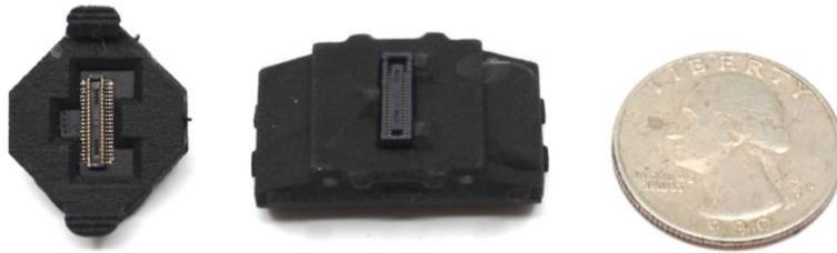
Figure 3- Mini logger bottom and mini-logger processor top with 110 mAh battery
