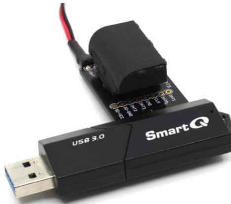
**Figure 9- Processor top with USB portable card reader for 3<sup>rd</sup> party data upload**
